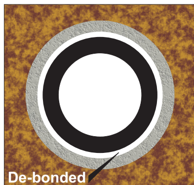
Debonding at cement/casing interface.
